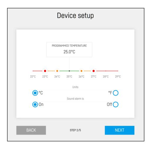
When the temperature exceeds the set range (default is 24°C - 26°C), it turns on corresponding circuit (heating when it's too cold or cooling when it's too hot). When the temperature exceeds the red limits the alarm will be triggered and you will be notified by sound alarm if you have turned it on. You will also get notified by email and push notifications.
