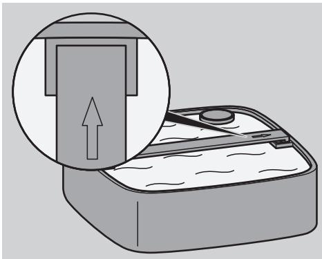
Arrows at the top edge of the filter case, on the filter media securing plate and on the filter baskets indicate the correct alignment.
