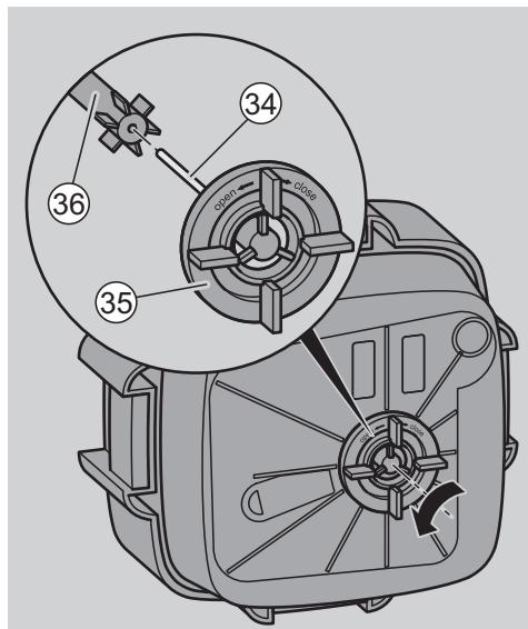
The impeller is on the bottom side of the motor head. The impeller is comprised of an impeller wheel (36) and an impeller shaft (34).
