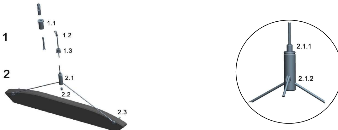
Pict. 1: Steel wire suspension aquafit 2 (art.-No. 80401)
